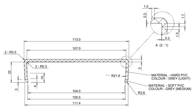
MATERIAL - AS NOTED COLOUR - AS NOTED EXTRUSION LENGTH - 5.0 Mtrs ACTUAL PANEL THICKNESS - 105.6mm
