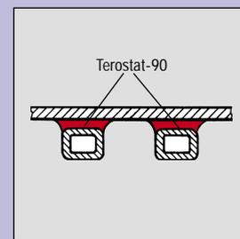
Bonding of side panels, roof and floor elements to load-bearing structures
