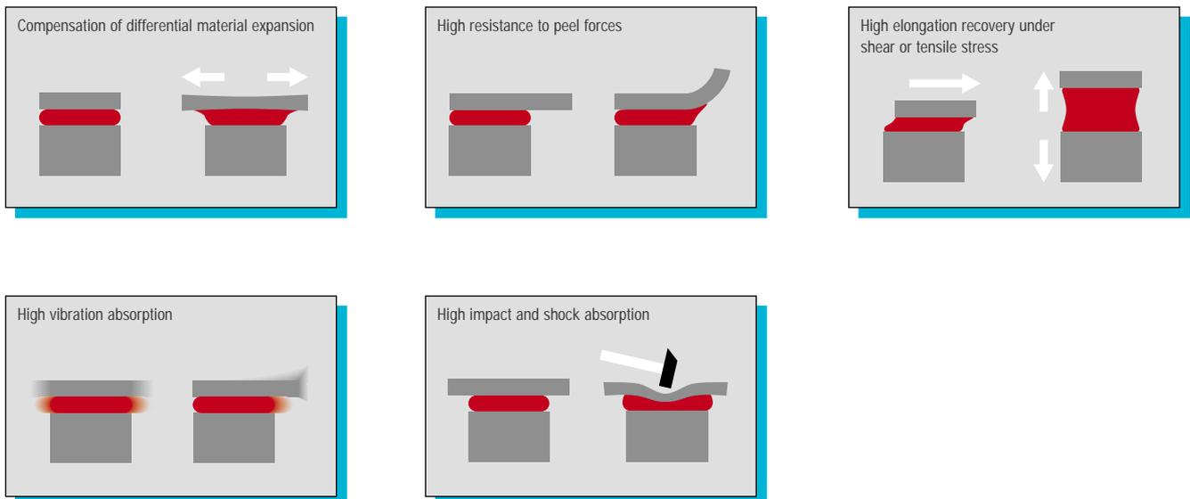
Figure 1: Advantages of elastic bonding and sealing
