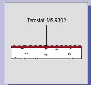
Coating to seal large porous surfaces
