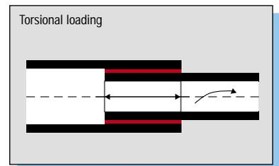
Thin-walled pipe lap or strap joints which are subjected to torsion can reach the same strength as the metals involved.
