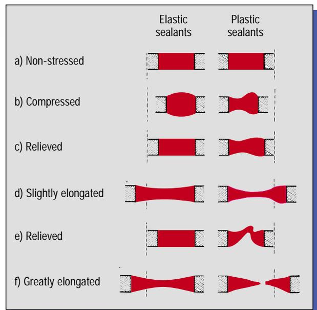
Figure 3: Behaviour of sealants under deformation
