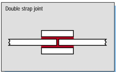
Provides better strength than a single strap, but is more complicated. Seldom used as none of the visible faces are plane.
