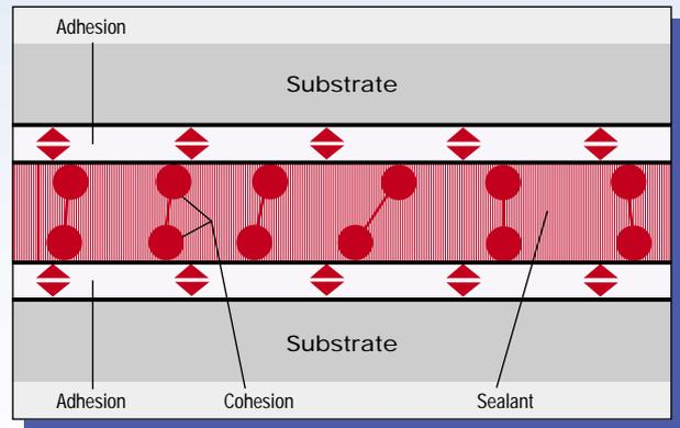
Figure 2: Functional mechanism of sealants
