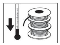
**To ensure optimum performance**, several important requirements should be noted prior to the installation of any Pressure Sensitive Adhesive (PSA) taped product. Be sure to store this product at 72°F (22°C) and 50% relative humidity. **DO NOT** apply when temperatures are below 60°F nor above 100°F, as this may affect the performance of the tape.
