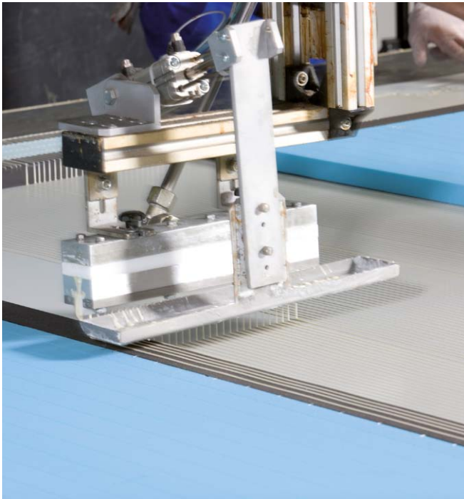
Figure 15: Application of a 2 component PU adhesive
