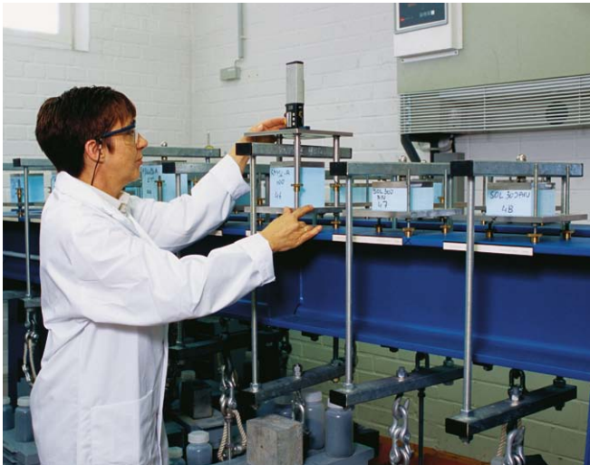
Figure10: Testing creep performance in Dow's dedicated laboratory
