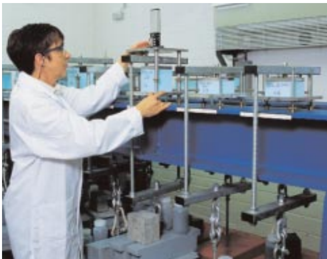
Fig. 10 Creep testing STYROFOAM in the laboratory
