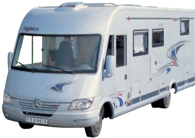
Fig. 17 Robust body consisting of floor, wall and roof panels with STYROFOAM core
