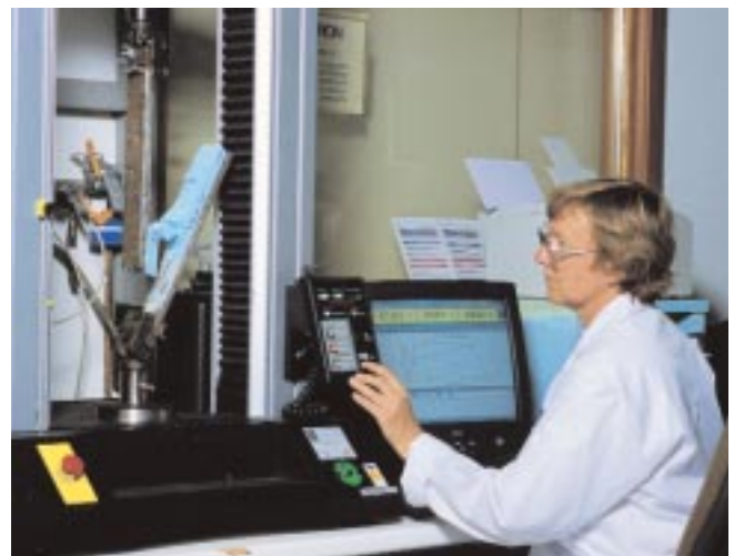
Fig. 11 Shear test on STYROFOAM
