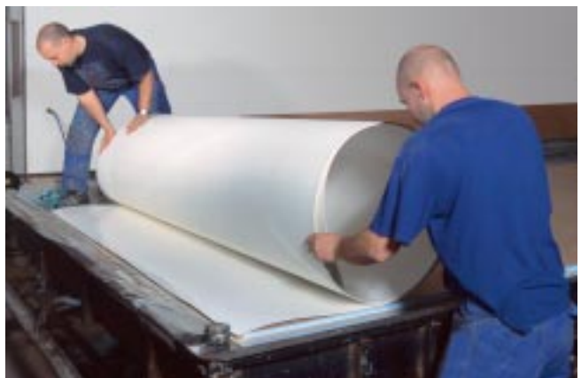
Fig. 9 Applying facing layer (GRP in this illustration)
