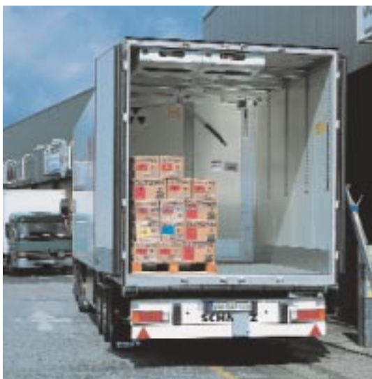
Fig. 14 Well insulated and able to support loads: refrigerated truck bodies using STYROFOAM cored panels.
